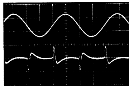
Fig. 2 — Scope photo showing the fundamental sine wave (top trace) and a typical crossover distortion waveform (bottom trace).
